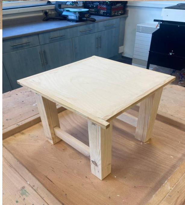
Ks4 Pics of a bench made by two students for the local army cadets group and a small bedside table made by Ellis Parr. Both using frame joints (Mortice & Tenon and Bridal) which is a focus area for students this term
